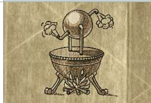
The “Aeolopile”: Heron of Alexandria developed an early type of steam engine in the 1 st century AD with his so-called “steamball”
